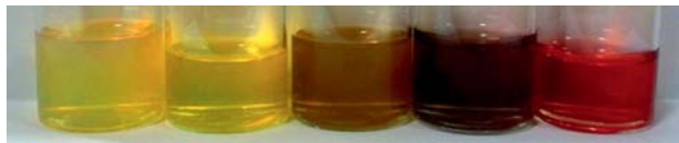
Figure 1. The Au, Ag and Au/Ag core-shell (Ag core-Au shell) colloidal suspensions were prepared by a modified Turkevich thermal co-addition of the sodium citrate solution to the auric acid and silver nitrate mixtures with the predetermined Au/Ag ratios of 100% Au, 75% Au: 25% Ag, 50% Au: 50% Ag, 25% Au: 75% Ag and 100% Ag. The solutions are displayed in the image above from the greatest silver content on the left (Ag 100%) to the greatest gold content on the right (Au 100%).
